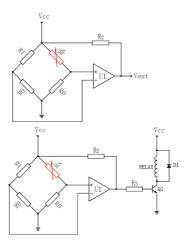
This is an ideal circuit for applications that require on-off switching at a specified force. It consists a Wheatstone bridge circuit and a voltage comparator.
