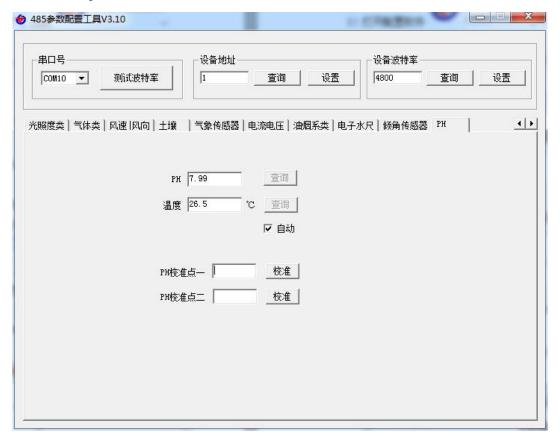
3) Put the pH electrode into a known pH standard buffer solution with pH<7 at room temperature (around 25  $^{\circ}$  C), enter the pH value of the standard buffer solution at the calibration point, and cancel the automatic when the value is stable, and click Calibrate Click "Calibration" to perform the first point calibration.
