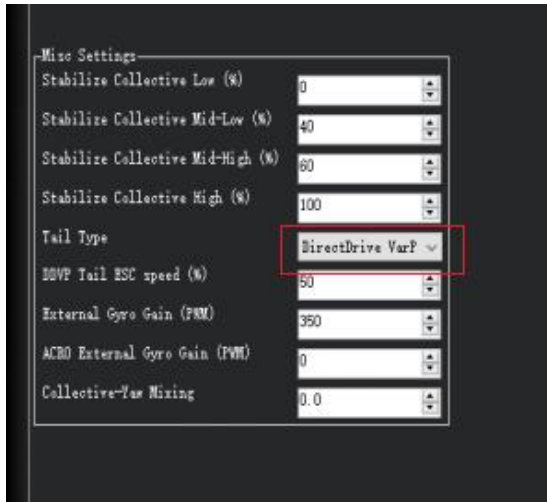
Figure 5 Select Direct Drive Variable Pitch (DDVP)
