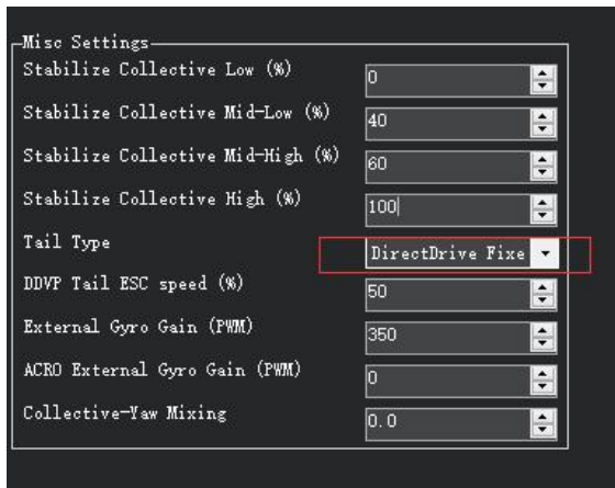
Figure 9 Select Direct Drive Fixed Pitch Counter-Clockwise
