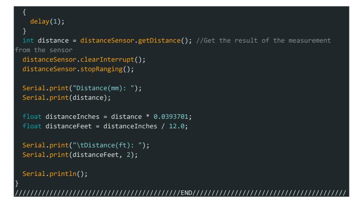
Opening your serial monitor to a baud rate of **9600** should show the distance between the sensor and the object it's pointed at in both millimeters and feet. The output should look something like the below image.
