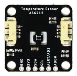
The AS6212 accepts a supply voltage between **1.7V** and **3.6** and typically consumes **6µA** during normal temperature conversions and **0.1µA** on standby. The AS6212 normally runs at **3.3V** and receives power either through the connectors or the dedicated **3.3V** and **GND** PTH pins.
