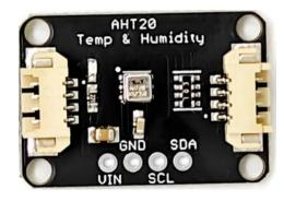
The AHT20 uses standard I2C so its easy to use with any Arduino or Linux/Raspberry Pi board. This sensor has a typical accuracy of +- 2% relative humidity, and +-0.3 °C. There is only one I2C address so its not a good option when you need multiple humidity sensors. The default I2C address is **0x38**. It cannot be changed.
