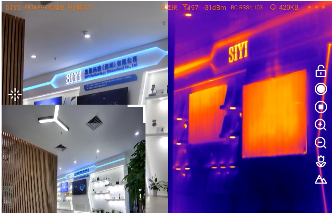
Main Window: Split Image – Zoom Camera & Thermal Camera
