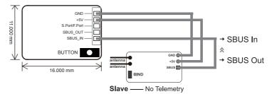
Smart Port (S. Port) is a signal wire full duplex digital transmission interface developed by FrSky Electronic Co., Ltd. All products enabled with Smart Port (including XJT module, XSR,X6R and X8R receiver, new hub-less sensors, new Smart Dashboard, etc), serial port user data and other user input/output devices can be connected without limitations for numbers or sequences at a high transmission speed.
